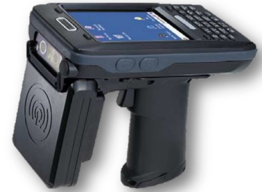
PDA with Gun Handle and Front Facing RFID Reader
