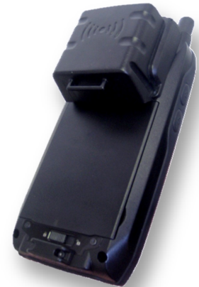
PDA with backpack RFID Reader
